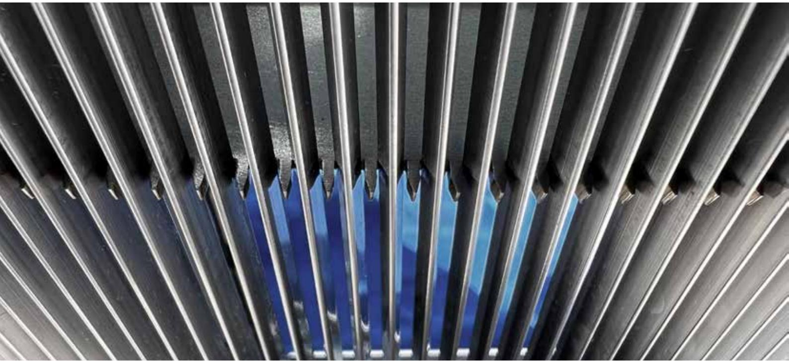
Precisely engineered rakes clean the bar array to ensure clog free operation without washwater or brushes.
